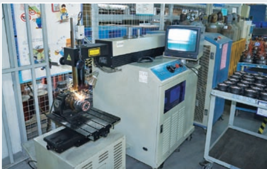
Automatic Laser Welding
